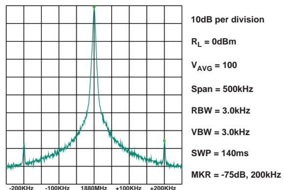
Figure 11. Output spectrum showing reference spurs.
