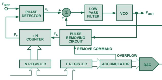
Figure 8. Fractional-N synthesizer.
