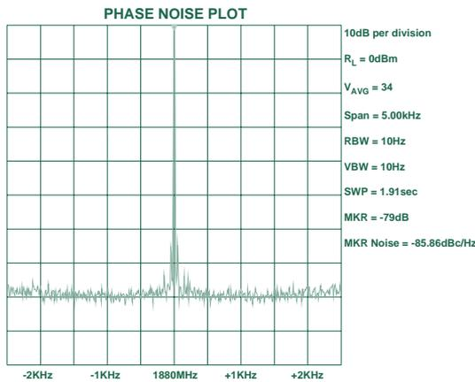
Figure 8. Typical spectrum-analyzer output.
