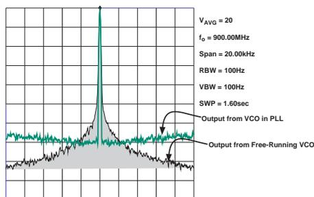
Figure 5. Phase noise on a free-running VCO and a PLL-connected VCO.
