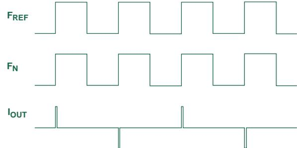
Figure 10. Output current pulses from the PFD charge pump.
