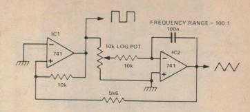
circuit is the basis of most function generators. By bending the triangle it is possible to synthesise an approximation to a sinewave. With a bit more electronics it is also possible to make the oscillator voltage controlled.
