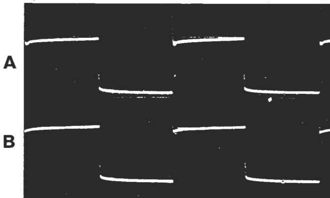
Fig. 2. A 2-volt spike on leading edge of waveform (A) is removed (B) by using a bypass capacitor from V_{cc} to ground.
