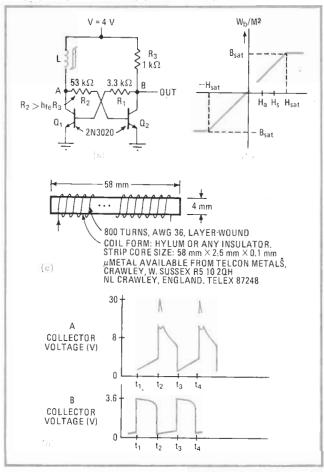
**Field sensitive.** Saturable core reactor enables oscillator to detect change in any magnetic field whose flux lines cut reactor windings (a). Oscillator frequency is determined by the core saturation time (b). Inductor is made of  $\mu$  metal, insulated core form, and 800 turns of high-gauge wire (c). Timing diagram details operation (d).
