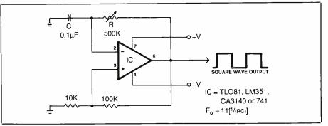
Fig. 1. Simple, low-cost multivibrator.
