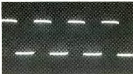
Fig. 1. Screen photo of a 10-volt peak-to-peak square wave from an old Heath Model IG-18 sine/square-wave audio generator.
