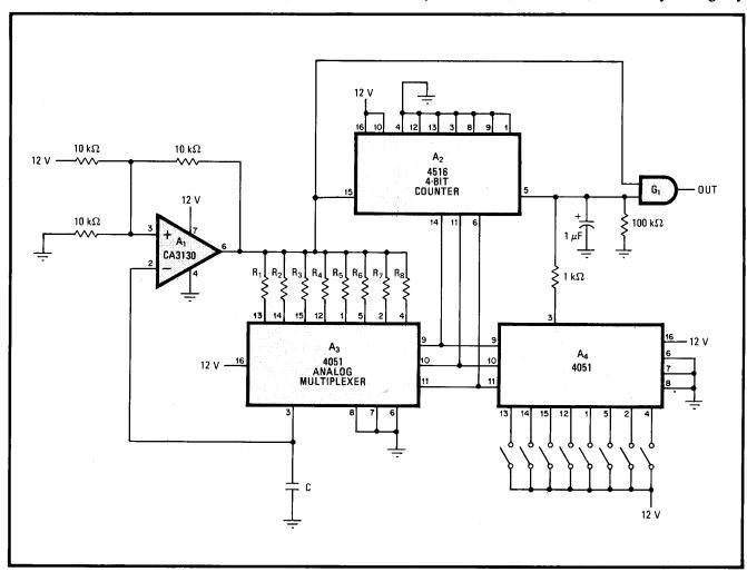
**Scanned tones.** Self-gating oscillator,  $A_1$ , advances counter and with aid of multiplexer  $A_3$  sequentially places  $R_1-R_8$  in series with C so as to control frequency. Op amp's high-input impedance and C-MOS output ensures high oscillator stability. No signal appears at output until a keyboard switch is closed, when  $A_4$  freezes counter and activates  $G_1$ , enabling generation of the single desired frequency.
