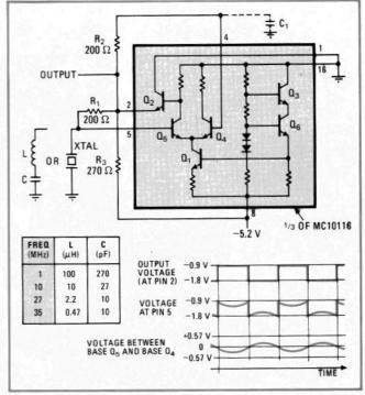
**Stable.** ECL-oscillator frequency, determined by crystal or LC tank circuit, is insensitive to variations in supply voltage. Capacitor  $C_1$  balances stray capacitances (e.g. from crystal holder) that might cause parasitic oscillations; its value is  $(R_1/R_2)C_{\rm stray}$ .
