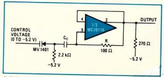
Voltage tuning. Varactor diode in place of C makes circuit a voltage-controlled oscillator. This VCO operates at (15 ±10) MHz.
