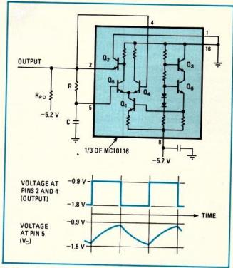
2. Operation. Circuit diagram shows how ECL oscillator operates. Output voltage is fed back to Q<sub>4</sub>. Capacitor voltage at pin 5 tries to reach voltage at pin 4, causing output to switch between different ECL levels. Oscillator can never hang up.
