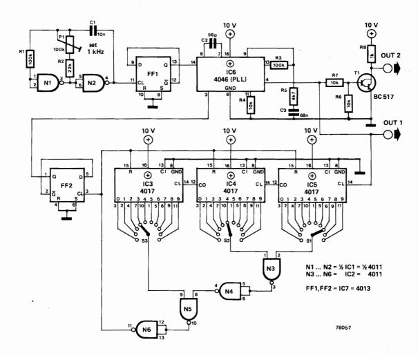
The output frequency of this squarewave generator can be programmed in 1 kHz steps from 1 kHz to 999 kHz. The heart of the circuit is a 4046 CMOS phase-locked loop which has an extremely wide capture range.
