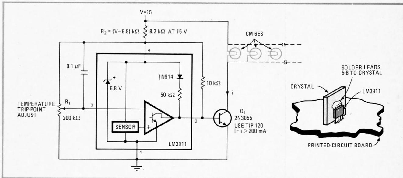
**Light adjustment.** Crystal oven uses low-cost pilot lamps for heat source, \$2 integrated-circuit temperature controller (left). Current through lamps, and thus temperature generated, is a function of the actual oven temperature and the temperature set by read:  $R_1$ . Temperature-critical elements of crystal oscillator should be placed close to LM3911 (right). Unused pins of LM3911 are soldered directly to crystal holder.
