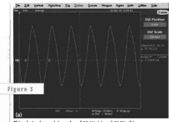
This photo shows duty cycles of 55.1% (a) and 65.3% (b).
