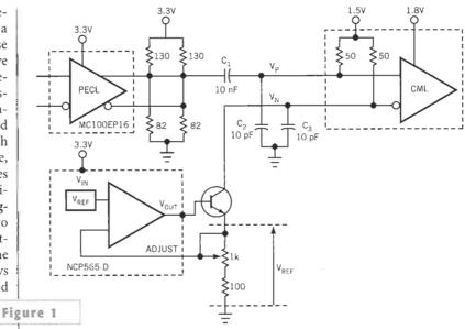
This circuit can make slight adjustments to the duty cycle you apply to a CML input.
