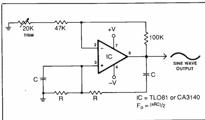
Fig. 5. Simple Wien-bridge oscillator gives relatively pure sine-wave output.
