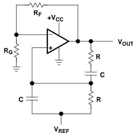
Figure A-37. Basic Wien Bridge Oscillator
