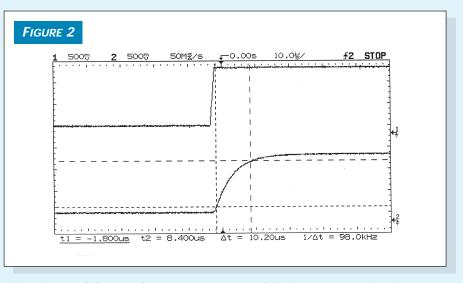
IC, in Figure 1 delivers a clean response to a modulation-input step function.
