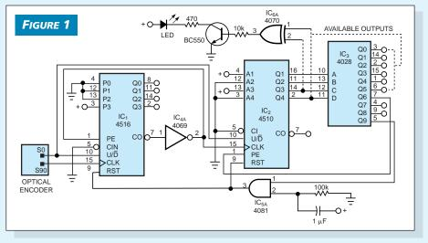
An optical encoder, immune to false switching, takes the place of a counter-controlled range switch.
