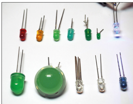
Figure 5. A LED miscellany. Top row, from left to right: red, yellow and four different green LEDs of 1970s vintage, compared to a modern blue LED which is so bright that its light saturates the camera sensor. Bottom row: modern green LEDs in 10 mm and 20 mm packages, and RGB, white and infrared LEDs.
