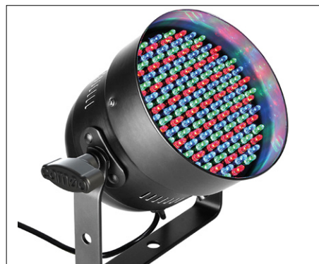
Figure 10. Cameo type CLP56RGB05PS PAR stage effect light with 151 colored LEDs and a power rating of around 30 W at 230 V. Not only does the light sport a DMX interface for remote control, it also has a built-in microphone to enable 'light organ' effects.
