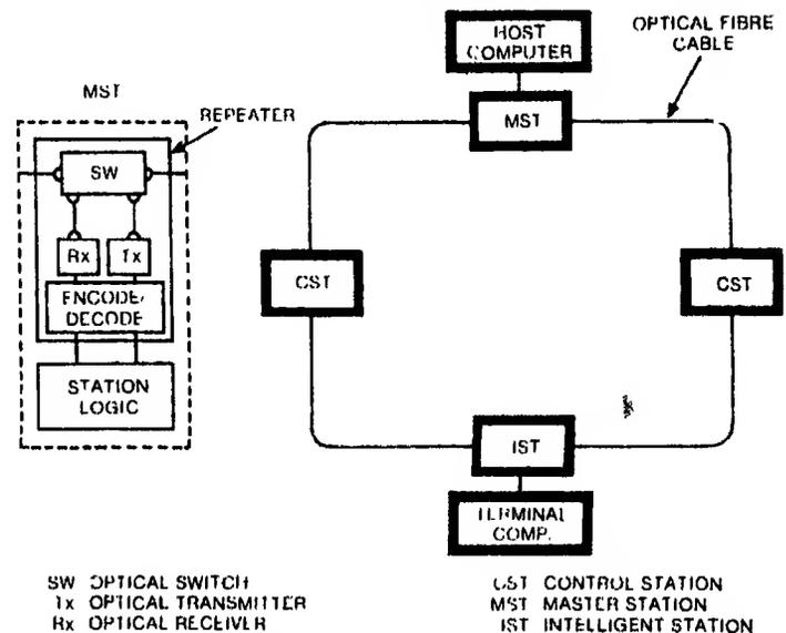
Fig. 6: Basic configuration of the DFW system.
