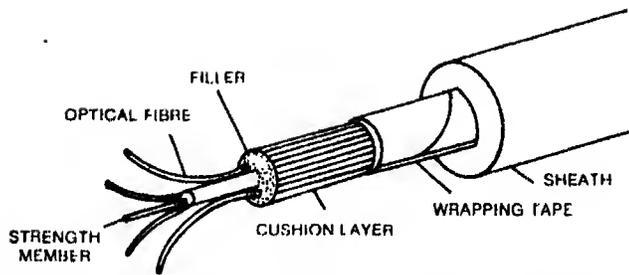
**Fig. 3: Long wavelength, four-core layer type optical fibre cable structure.**
