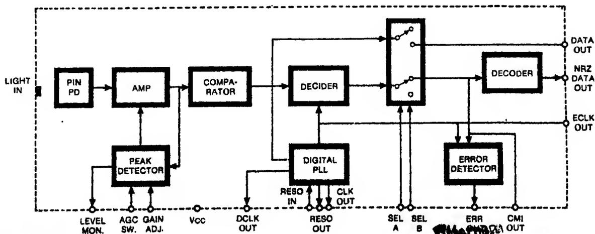
Fig. 2: Block diagram of receiver module.
