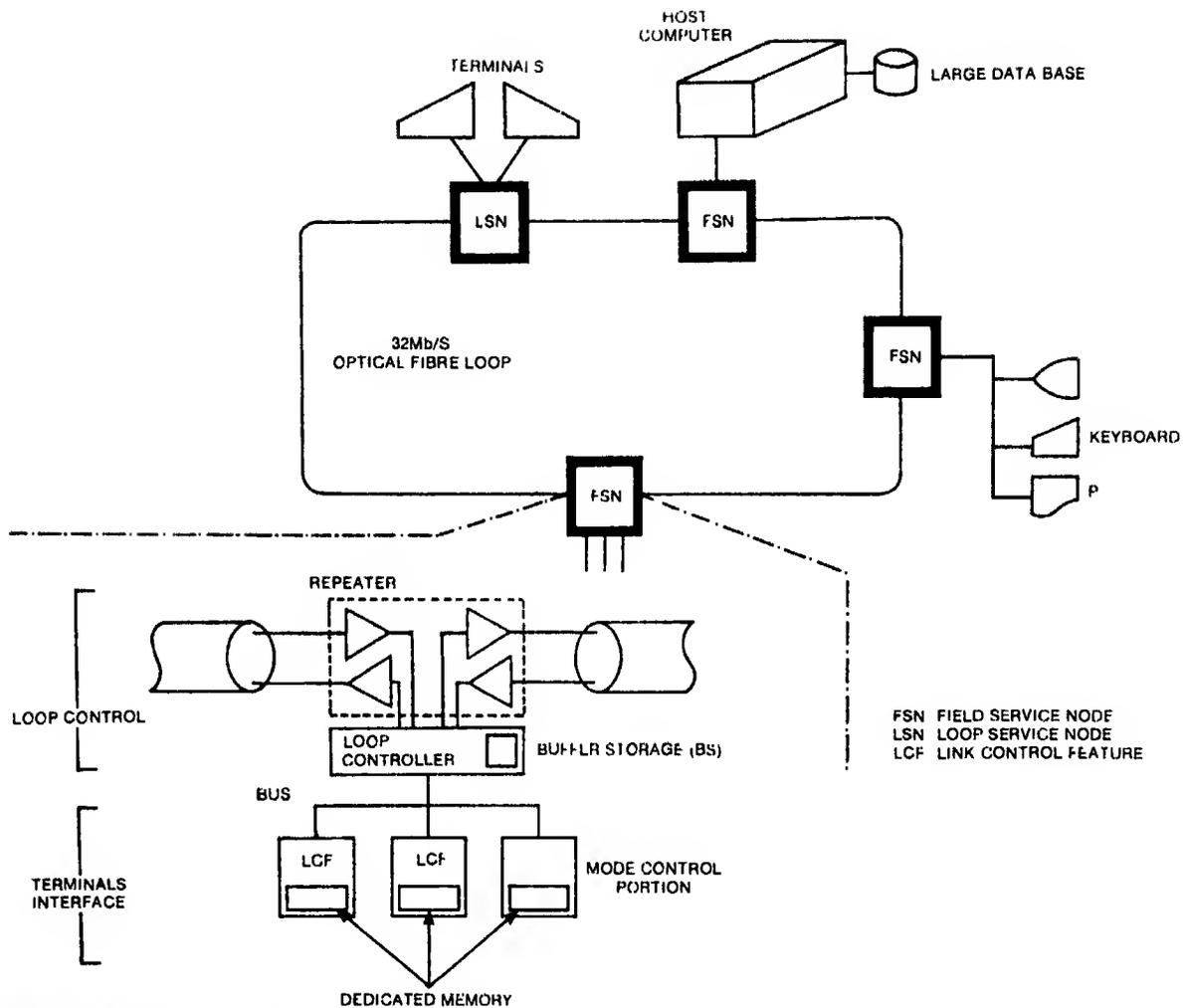
**Fig. 7: System configuration of 32MB/sec loop network.**
