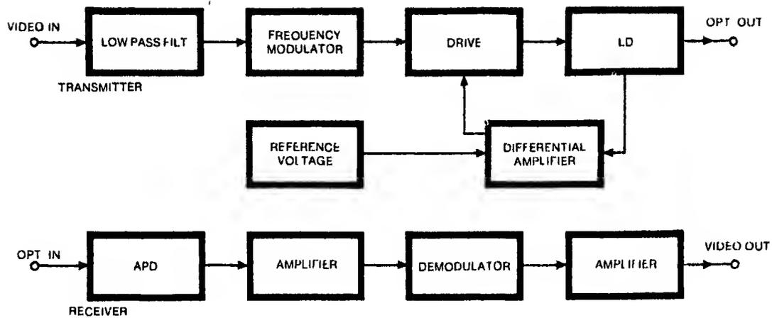
Fig. 5: PFM equipment configuration.
