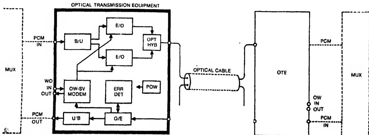
Fig. 4: Configuration of an optical digital transmission system.
