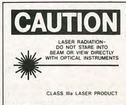
FIG. 8—ANY LASER DEVICE must contain warning labels according to the specific type of device. Our hand-held laser must display this warning, in addition to a label stating that it conforms to specifications and a warning at the laser aperture.
