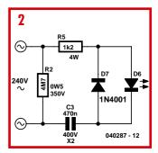
A metal film resistor should not be used for R1. With a value of 1.2  $k\Omega$  the peak dissipation will be nearly 100 W for a period of a few hundred microseconds: carbon film resistors are better able to withstand this treatment. The most tolerant are the ceramic wirewound types: the small 4 W versions are suitable. Even if a value of 680  $\Omega$  is used, the ceramic 4 W types are preferred. Resistors rated at less than 0.5 W generally do not have a sufficiently high working voltage.
