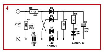
LED itself takes 33 mW. The overall efficiency is thus considerably improved: at 51 mW only 60 % of the total power is lost to heating the environment.
