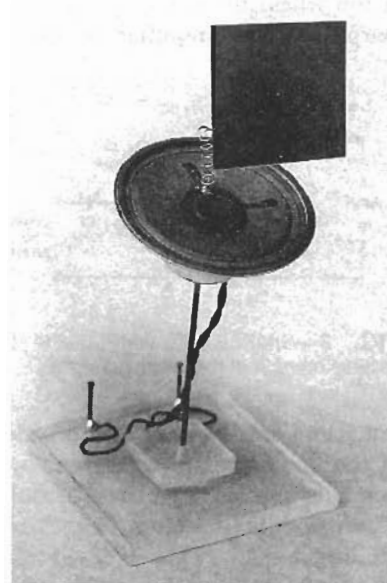
FIG. 1—A SPEAKER MODULATOR using flex-wire for positioning, and a small speaker with cone still intact.
