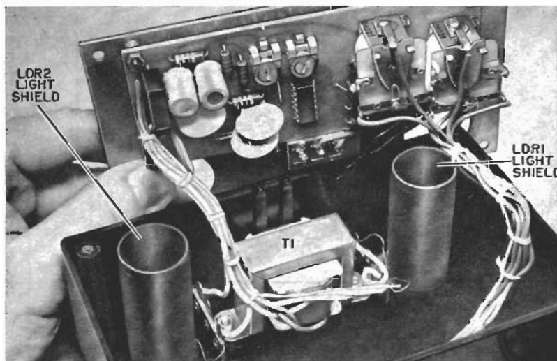
All components except power transformer, on/off switch, and LDR's mount on printed circuit board. Spacers and 4-40 machine hardware fasten circuit board to case top.
