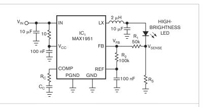
Figure 3 Adjusting the feedback signal improves the efficiency in this buckconverter driver for high-brightness LEDs.
