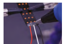
Above ♦ It takes just three solder joints to connect the LED strip
