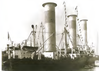
The three-rotor ship “Barbara” in Barcelona harbour, 1927. It suffered the ignominy of being sold and having its three rotors removed, converting to standard propulsion! https://commons.wikimedia.org/w/index.php?curid=48364872
