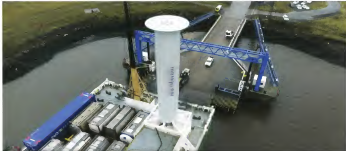
In this view, the Estraden is docked at the ro-ro terminal in Teesport, UK. The Flettner sails (one forward, one aft) are kept spinning, albeit at a much slower speed, providing the ship with some stability while vehicles driving on or off. At sea, the speed is significantly increased. We've seen figures of 300+ RPM although this has been difficult to verify.
