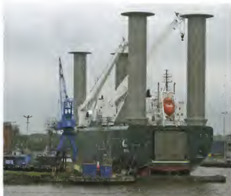
The four 27m x 4m Flettner Sails on the E-Ship 1, a 13,000t RoLo cargo ship that made its first voyage with cargo in August 2010. The ship is owned by the third-largest wind turbine manufacturer, Germany's Enercon GmbH and is used to transport wind turbine components. Maximum rotor speed appears to be in the order of 310 RPM, though this depends on both ship speed and wind direction/speed. (Courtesy Enercon GmbH).
