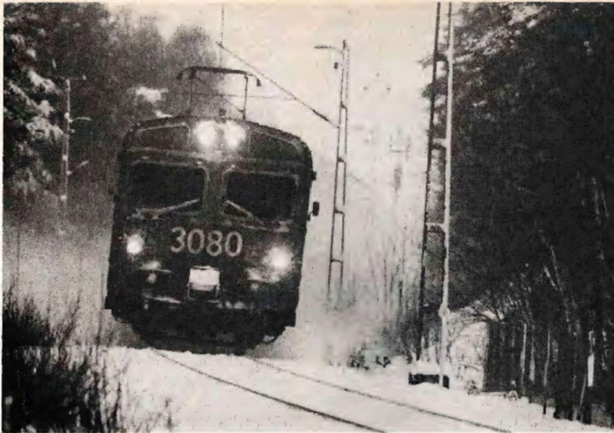
Fig.4: the Swedish electric BoBo locomotives operate in very cold conditions. Wet snow on the high-voltage (15kV) insulators is a constant problem for the engineers. (Photo SJ).
