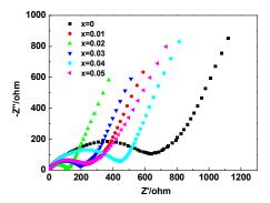
Fig. 9. Electrochemical impedance spectra of LiFe(PO<sub>4</sub>)<sub>1-x/3</sub>F<sub>x</sub>/C(x=0, 0.01, 0.02, 0.03, 0.04) cathodes at 25°C (amplitude is 5mV in the frequency range of 10<sup>5</sup>Hz~0.01Hz)
