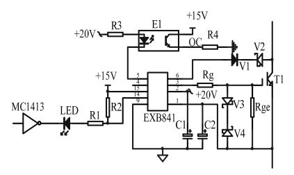
Fig. 9. IGBT drive circuit
