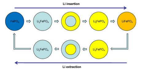
Fig. 4. Complete Li insertion and de-insertion cycle of a spherical LiFePO<sub>4</sub> particle.
