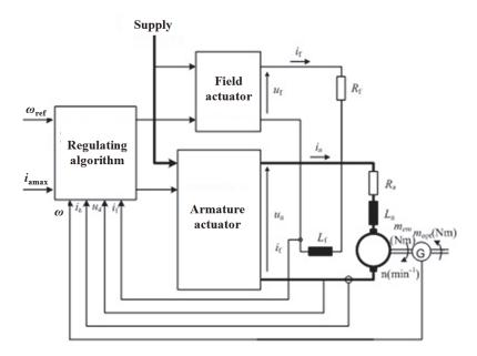
Fig. 9. Circuit for speed regulation of DC motor with independent field
