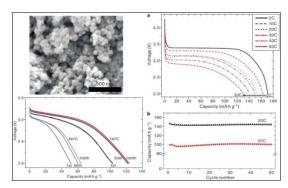
Fig. 10. The high rate performances of nano-sized LiFePO<sub>4</sub> (Kang & Ceder, 2009)
