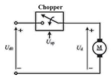
Fig. 7. Simplified presentation of the chopper supply of a DC motor Chopping frequency is by the definition:
