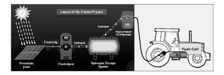
Fig. 20. "Hy-Tractor": Project layout with photovoltaic plant.
