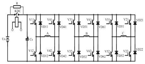
Fig. 8. Schematic Diagram of Power converter in Electrical Vehicle
