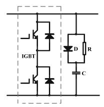
Fig. 12. IGBT snubbed elctronic circuit.
