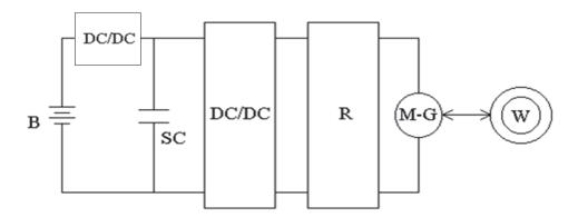
Fig. 5. Scheme of electrical drive vehicle with supercapacitor with possibitlity for using breaking energy; B – one-way voltage source, SC – supercapacitor; DC/DC – direct voltage converter; R – regulator; M-G – engine – generator (depending on working regime; W – drive wheels
