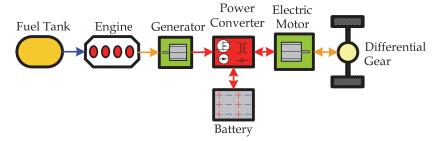
Fig. 8. Architecture of series HEV
