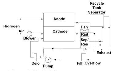
Fig. 22. Schematic diagram of the Fuel Cells System.
