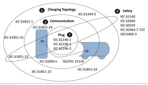
IEC 62196-1: Plugs, socket-outlets, vehicle couplers and vehicle inlets Conductive charging of electric vehicles, Charging of electric vehicles up to 250 A a.c. and 400 A d.c.
