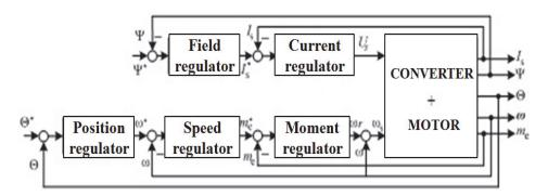
Fig. 10. Block diagram of AC motor regulator
