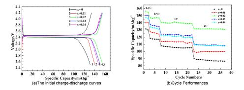
Fig. 8. The electrochemical performances of  $LiFe(PO_4)_{1-x/3}F_x/C(x=0, 0.01, 0.02, 0.03, 0.04)$
