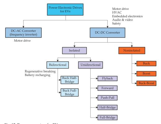
Fig. 15. Power converters for EVs
