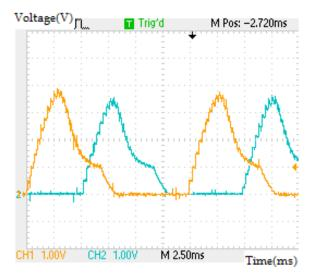
Fig. 19. Winding current waveform of n=500r/min under loaded 72Nm
