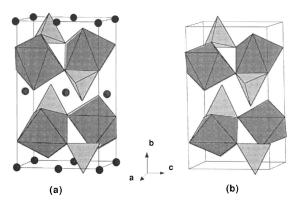
Fig. 3. Crystal structure of (a) LiFePO<sub>4</sub> and (b) FePO<sub>4</sub>
