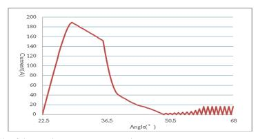
Fig. 3. Profile of designed SRM current vs. angle
