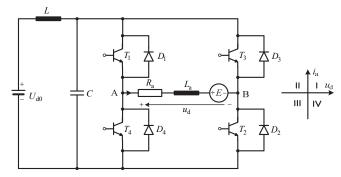
Fig. 8. Transistor bridge
