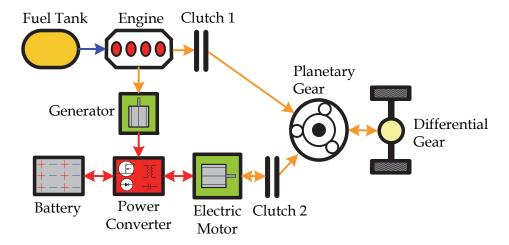
Fig. 11. Architecture of series-parallel HEV
