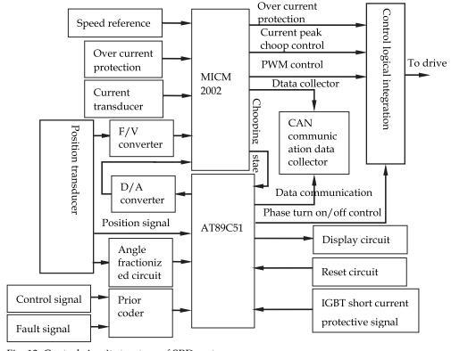
Fig. 13. Control circuit structure of SRD systems
