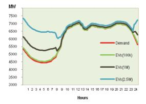
Fig. 3. Electric vehicles contribution to the consumption diagram leveling
