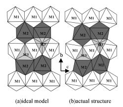
Fig. 2. Crystal structure of LiFePO<sub>4</sub> (a) ideal model and (b) actual structure.
