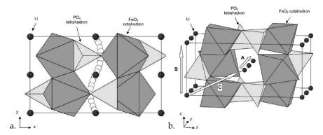
Fig. 5. Curved trajectories for Li ion migration between sites in the [010] direction. The diffusion path lies out of the *x-y* plane. (a,2D model. b,3D model, A, B, C denote [010], [001], [101] direction respectively)
