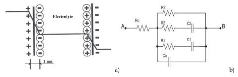
Fig. 2. (a) Cross section through a practical electrochemical double layer capacitor and profiles of the potential across an electrochemical capacitor; (b) Simplified equivalent electric circuit for an electrode – electrolyte interface
