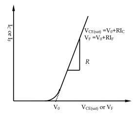
Fig. 11. Positive output characteristic curve of power devices
