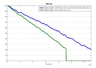
Fig. 30. SoC (%) analysis: Comparison of proposed HEV (blue) and pure battery EV (green).
