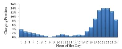
Fig. 14. Expected charging profile for uncontrolled charging scenario
