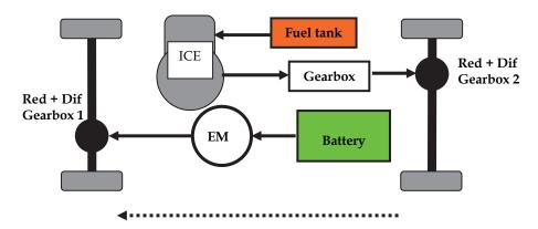
Fig. 12. PHEV without Generator
