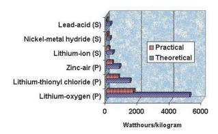
Fig. 8. Energy density in various battery chemistries
