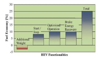
Fig. 10. Fuel saving components of HEV in city transport
