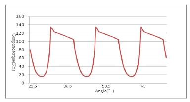
Fig. 4. Profile of designed SRM composed torque vs. angle
