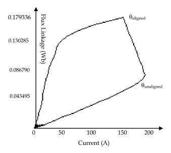
Fig. 2. Profile of designed SRM flux-linkage-current
