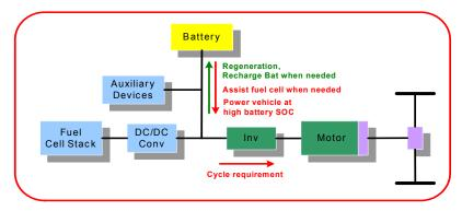
Fig. 16. Fuel Cell Hybrid Electric Vehicle configuration
