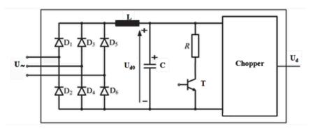
Fig. 6. Principal scheme of chopper supply
