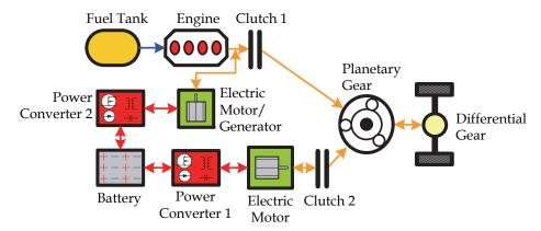
Fig. 12. Architecture of complex HEV
