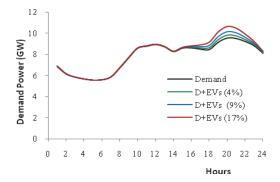
Fig. 4. Load profile simulation of the peak demand weak for year 2015 with 4, 9 and 17% light duty fleet replacement with EV's that recharge at peak hours in Portugal mainland.
