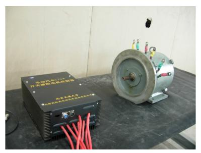
Fig. 23. SR drive system for EV
