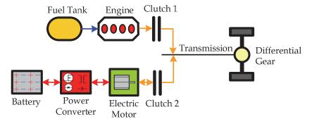
Fig. 10. Architecture of parallel HEV
