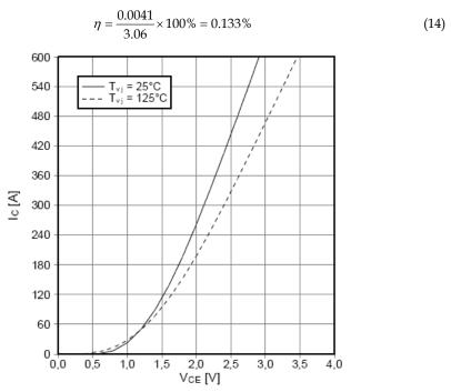
Fig. 10. IGBT BSM300GA120DLC output curve under different voltage
