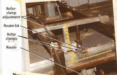
The router system designed by the contracting company had an unguarded router bit and a board-hold-down mechanism that required frequent adjustment. The router could only be powered off by unplugging it, so the operator adjusted it while bit was spinning. His wrench slipped, and his hand hit the spinning blade.
