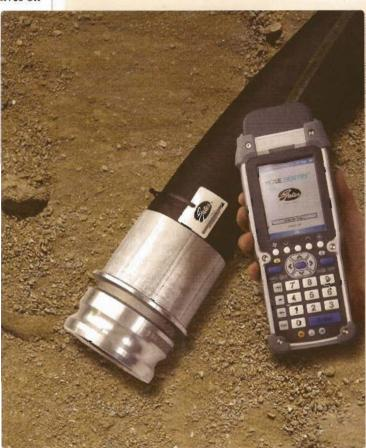
RFID tags speed and simplify hose-assembly identification. Technicians scan the tag using a PDA with an RFID reader, which then displays information such as the type of hose, end fittings, and length.
