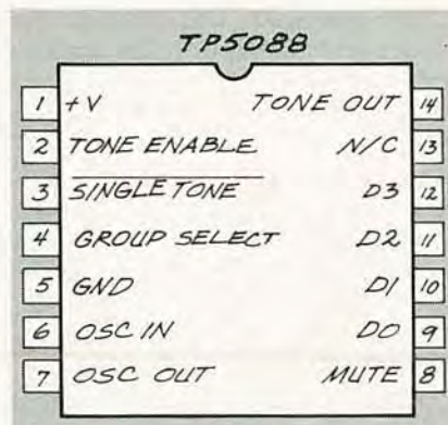
FIG. 1—THE 5088 DTMF GENERATOR is designed to be used under microprocessor control and, instead of the eight lines normally needed for keypad control, the digit is sent as four-bit binary information to the four data inputs.
