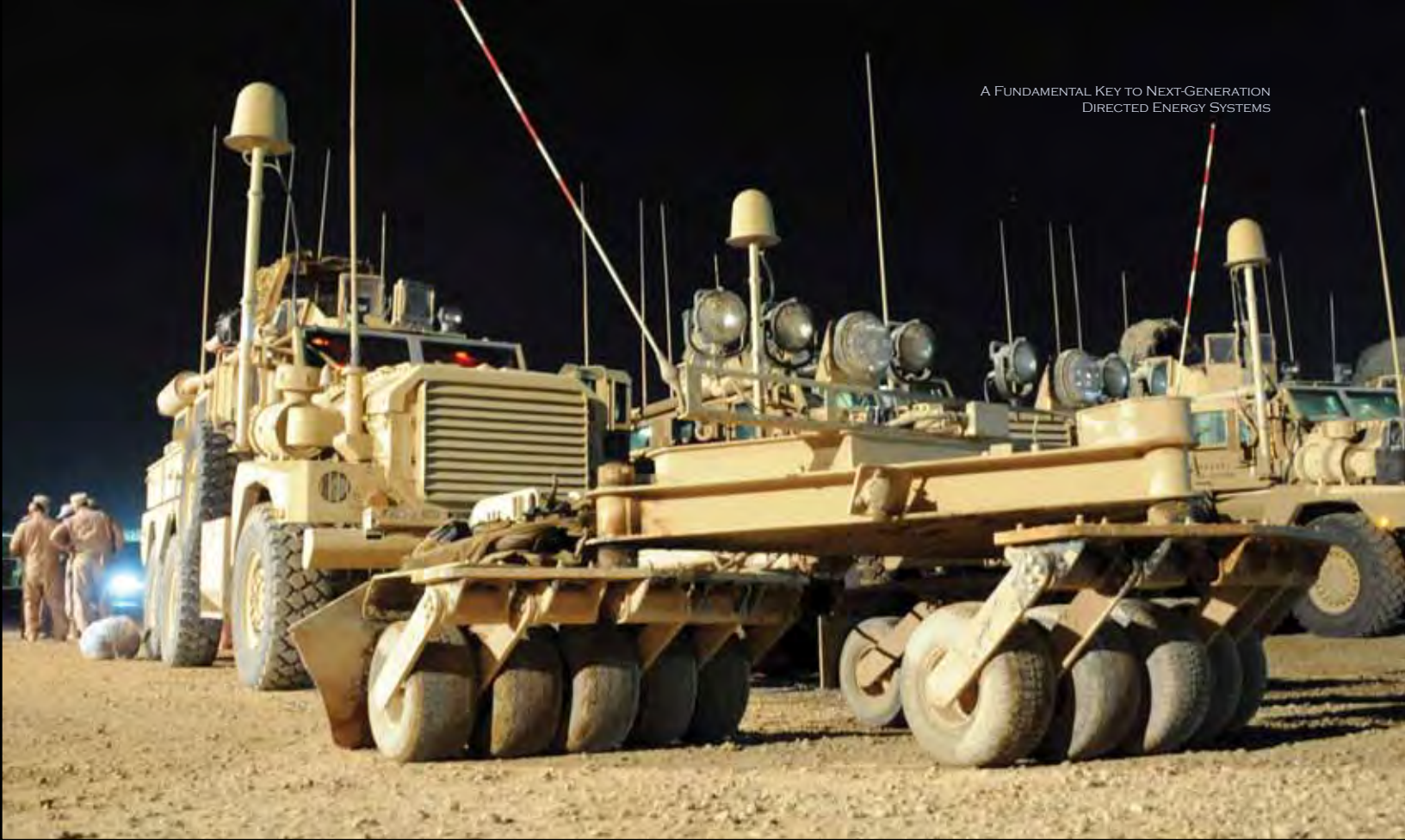
081107-N-1120L-072 RAMADI, Iraq (7 November 2008) Joint EOD Rapid Response Vehicles (JERRVs) assigned to Naval Mobile Construction Battalion (NMCB) 7's convoy security element are secured following an escort mission from a forward operating base. The Cougar-type JERRVs are employed by coalition forces for escort and logistics missions, and to protect personnel from IEDs. NMCB 7 is deployed to U.S. Forces Central Command to provide contingency construction support to coalition forces in support of Operations Enduring Freedom and Iraqi Freedom. (U.S. Navy photo by Mass Communication Specialist 2nd Class Michael B. Lavender/Released)
