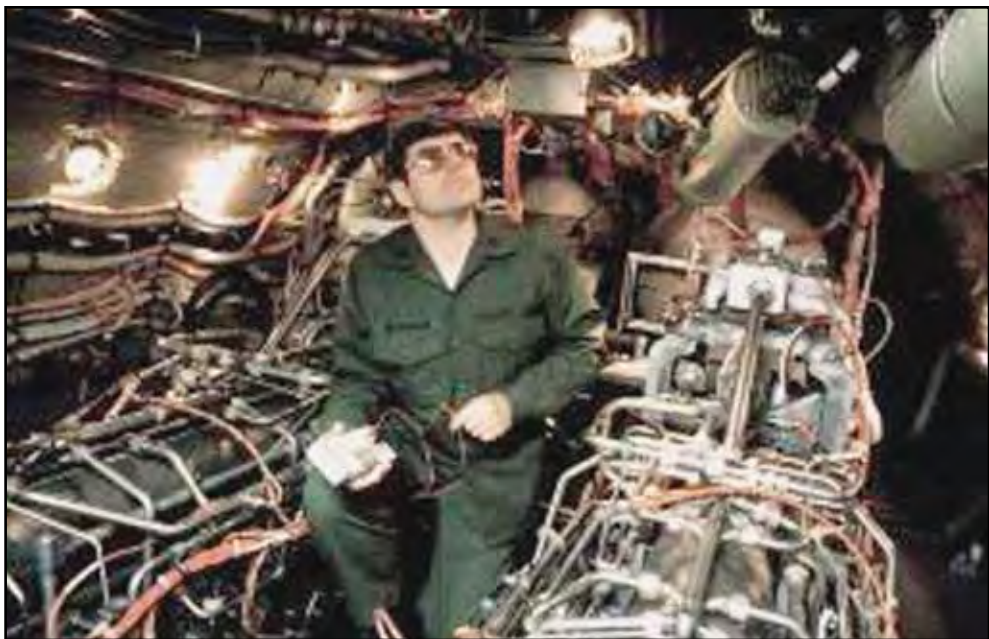
Figure 4. A laser engineer inspects a gas dynamic laser after installation aboard an NKC-135 airborne laser laboratory.
