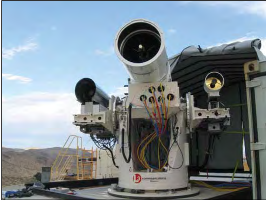
Figure 3. Photo of LaWS During Testing at the Naval Weapons Center, China Lake
