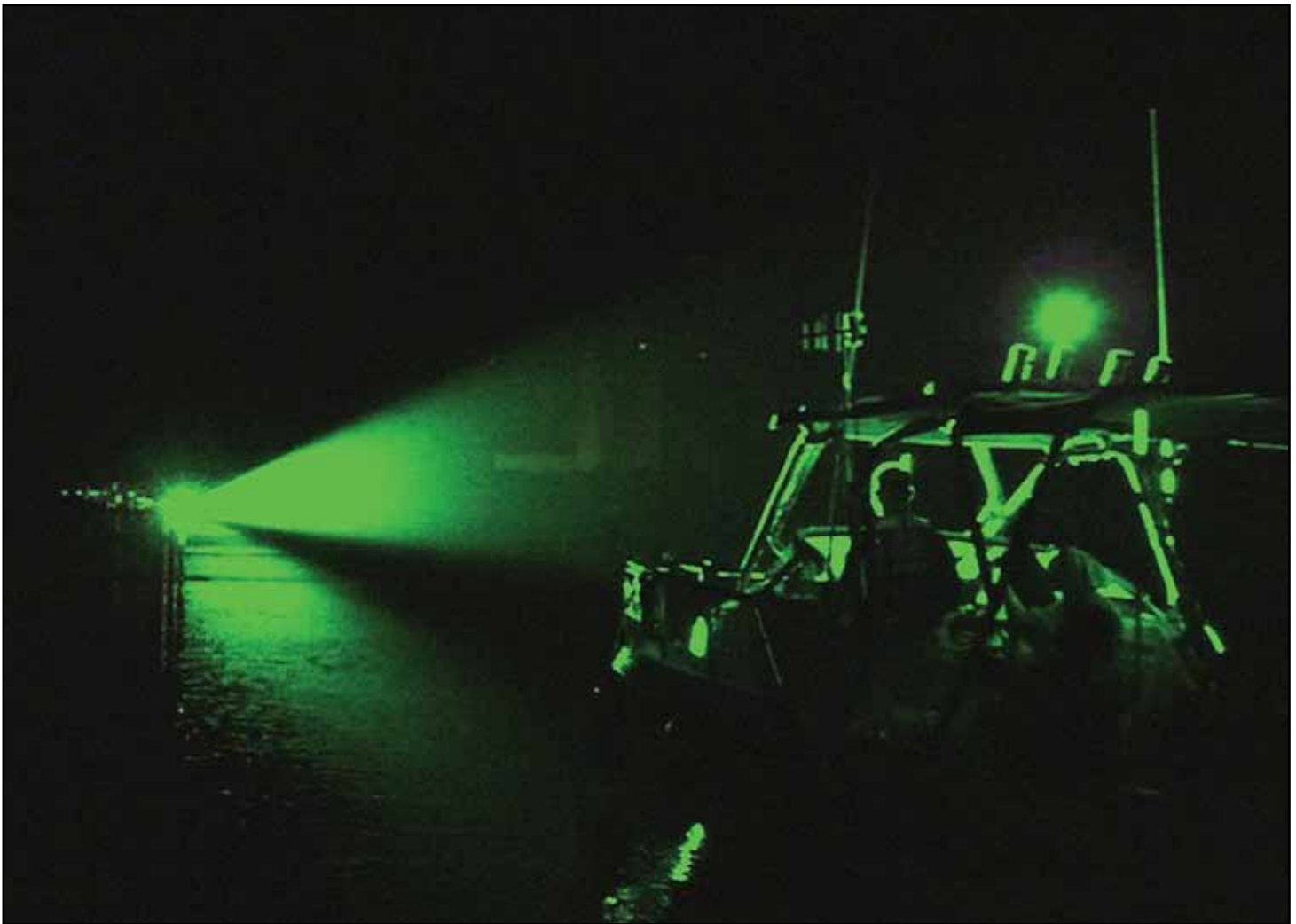
Figure 2. NAMRU-SA personnel execute operational field test at Kennedy Space Center, July 2009, in which a nonlethal laser prototype is evaluated for power delivery (stability and beam propagation) at range and human visual effectiveness aboard a maritime target.
