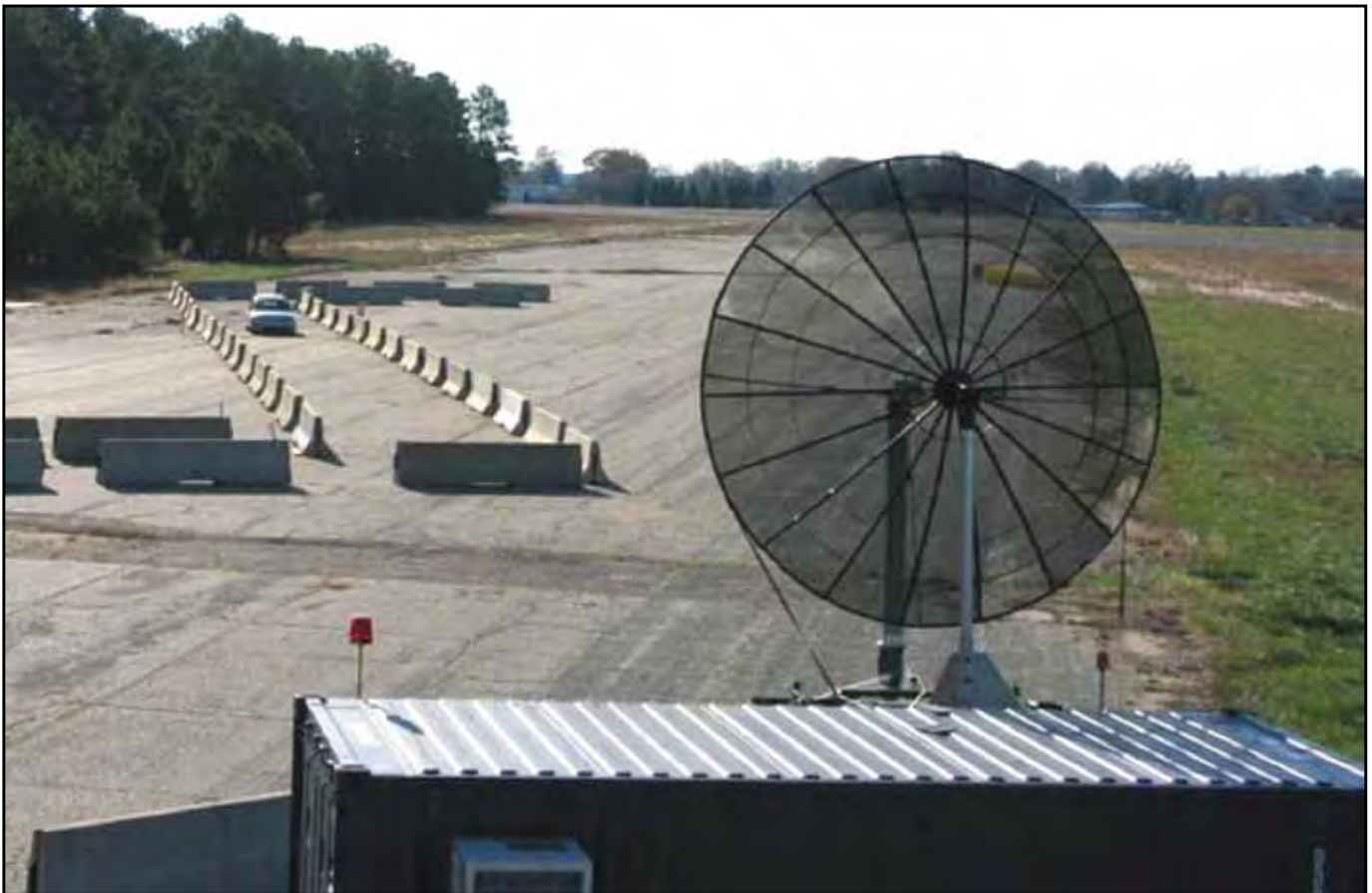
Figure 3. Multifrequency RF Vehicle-Stopper (RFVS) System
