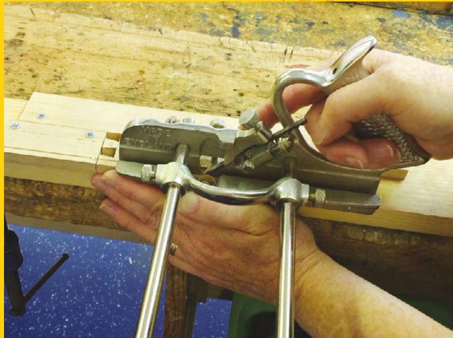
Above ✕ This is a plough plane: use it to carve grooves for the box lid to slide into
