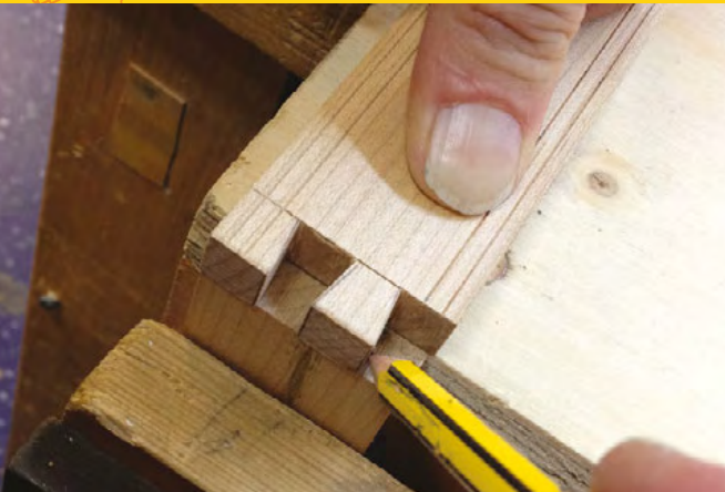
Above ♦ Marking out the sockets, following the lines of the dovetails
