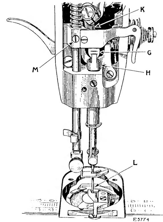
FIG. 7. SHOWING NEEDLE AND OSCILLATING HOOK CORRECTLY TIMED
