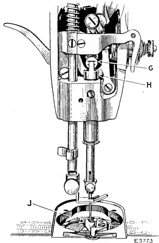
FIG. 6. SHOWING CORRECT ADJUSTMENT OF TIMING GAUGE
