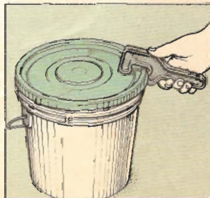
2 Premixed joint compound is the best choice for most work. Buy an inexpensive cover tool to open the 5-gal. buckets.
