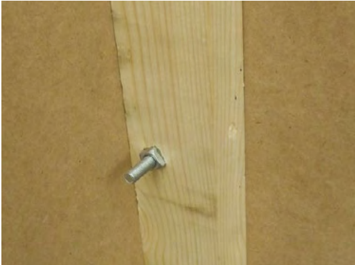
Above ♦ The joints holding the smoke chamber together. The bolt through the long side makes it easy to take apart for easy storage
