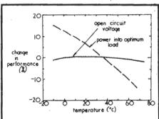
Fig. 1. Graph of pacemaker battery performance against temperature.
