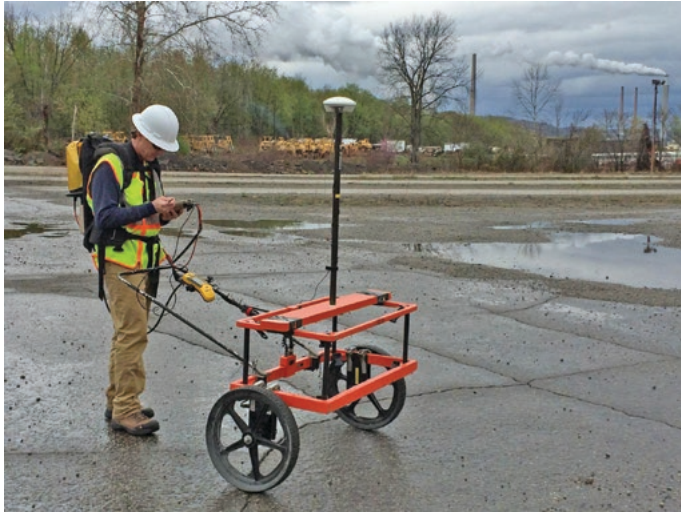
Fig.35: a Geonics EM-61 time domain metal detector. Note the GPS antenna. Source: GeoView Inc.
