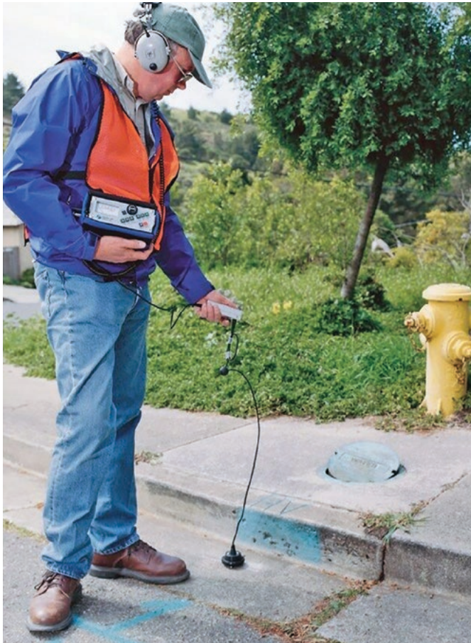
Fig.23 (left): a SubSurface Leak Detection ( www.subsurfaceleak.com ) LD-12 instrument in use. Such equipment is also used to trace utility pipes when a pulse wave generator device is connected.
