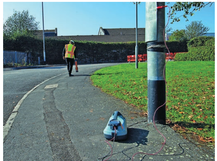
Fig.4 (right): the RD5100H2O+ at work, with the transmitter connected to a utility and handheld receiver unit in the background. Presumably, the Earth wire is being traced as the transmitter is connected to the body of the metal pole. The transmitter can also be used in an inductive mode, with or without a clamp.
