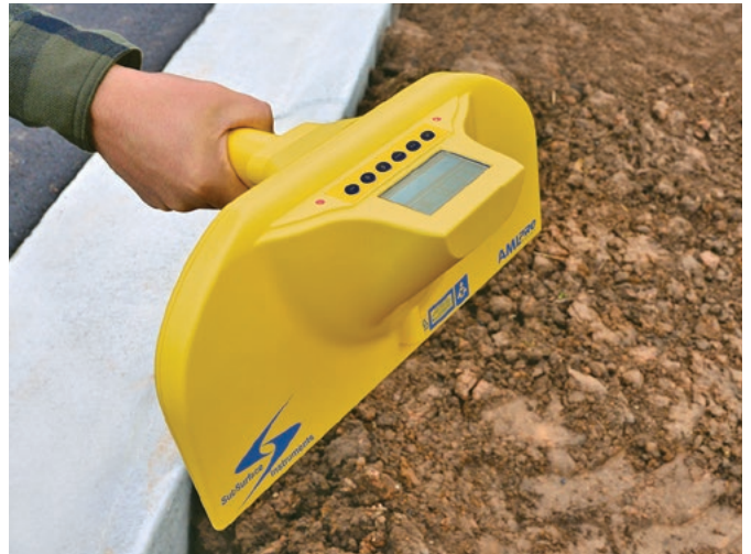
Fig.10: the AML Pro uses a 2.45GHz beam and is said to be able to find plastic pipes or any buried object that has an edge, including metal pipes.
