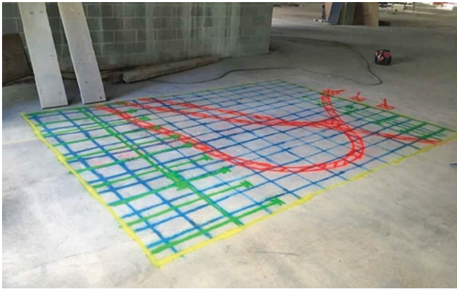
Fig.13: a concrete slab marked with the location of rebar and conduit, found with GPR. Image from www.ladsqld.com.au/services/concrete-scanning
