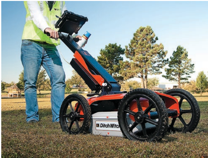
Fig.9: a typical Ground Penetrating Radar (GPR) machine in operation. It is pushed along the ground like a lawnmower, and data is recorded as a function of position.
