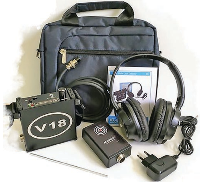
Fig.24 (below): the relatively inexpensive V18 water leak detector ( http://etowos.com/ ). See the videos titled “Acoustic Water Pipe Leak Detector +905414883700” at https://youtu.be/QCaoX3Bfu2w and “V18 Water Leak Detector” at https://youtu.be/_wxJkkjt1hc
