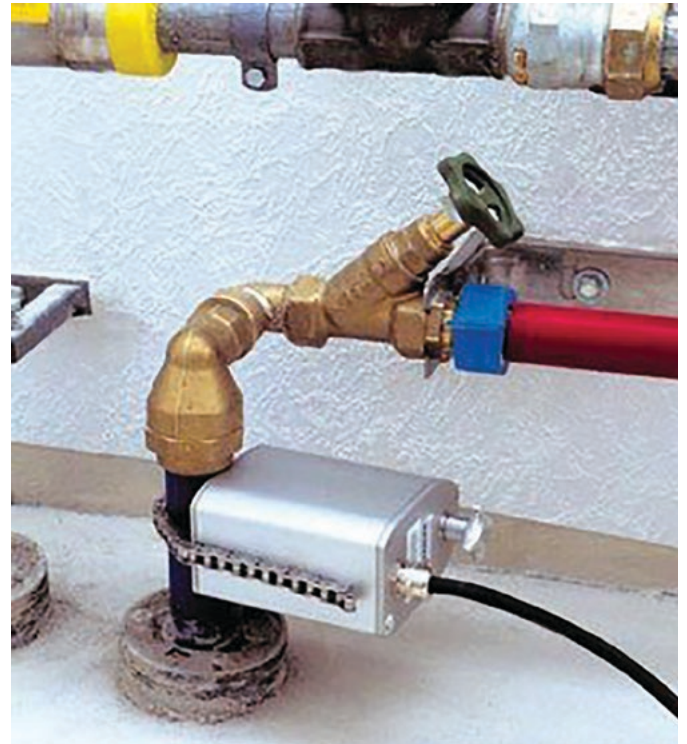
Fig.22 (right): a Sewerin "Knocker" which attaches to the outside of a plastic or other pipe with a chain and makes a knocking sound of adjustable frequency and intensity. This is conducted along the pipe and can be detected above ground. No water is released.
