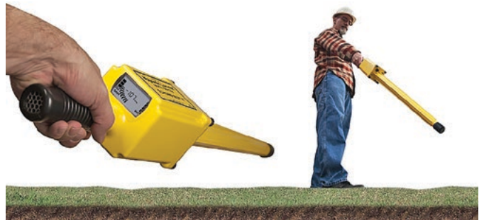
Fig.12: a handheld magnetometer, the Schonstedt GA-72Cd Magnetic Locator. This can be used to find UXO, and the military version is also used in de-mining operations in war zones. It looks for ferrous materials and does not respond to aluminium, brass or copper.
