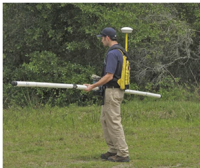
Fig.34: a Geonics EM31-MK2 ground conductivity meter, which operates at 10kHz. Source: GeoView Inc. Compare this with the build-it-yourself “Incredibly Sensitive Magnetometer” which we published in the December 2018 issue ( siliconchip.com.au/Article/11331 ).
