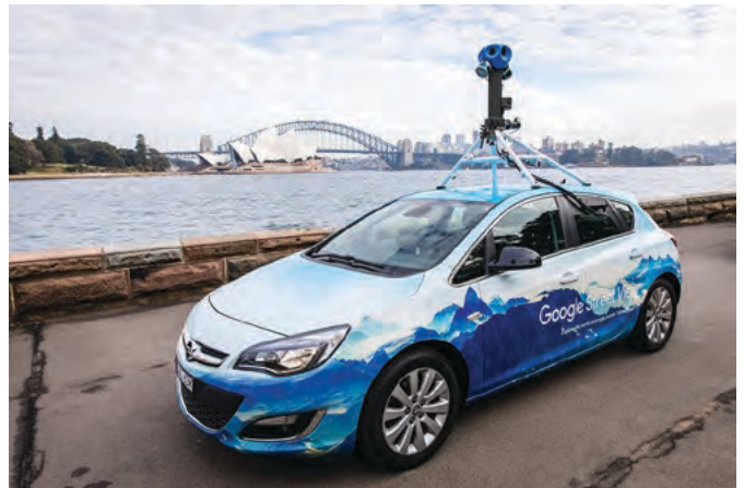
Fig.12: a Google Street View car in Australia. Note the cameras on top of the mast and the two LIDAR devices beneath the blue camera housing.
