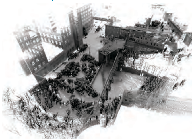
Fig.13: a typical image as produced by the company “Real Earth” using a Velodyne LIDAR “Puck LITE”, the same type said to be used on Google Street View cars. This 3D imagery can be used for guidance by autonomous vehicles such as cars and drones. Google also produces photographic imagery and other data.
