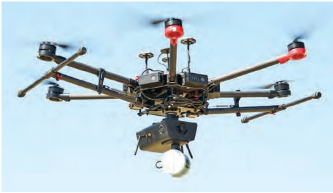
Fig.28: a drone with the Hovermap payload attached (the black box at the bottom with a white LIDAR device). Image courtesy CSIRO.
