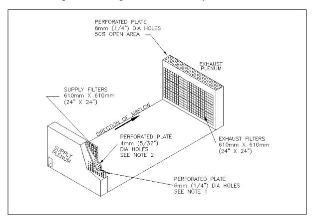
Figure 10-2. Hangar door and exhaust plenum details.
