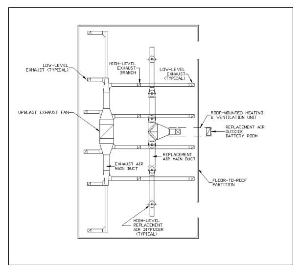
Figure 8-1. Ventilation system for battery maintenance facilities.
