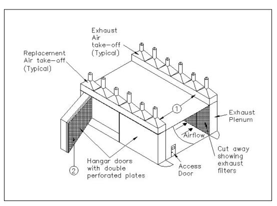
Figure 10-1. Crossdraft corrosion control hangar.
