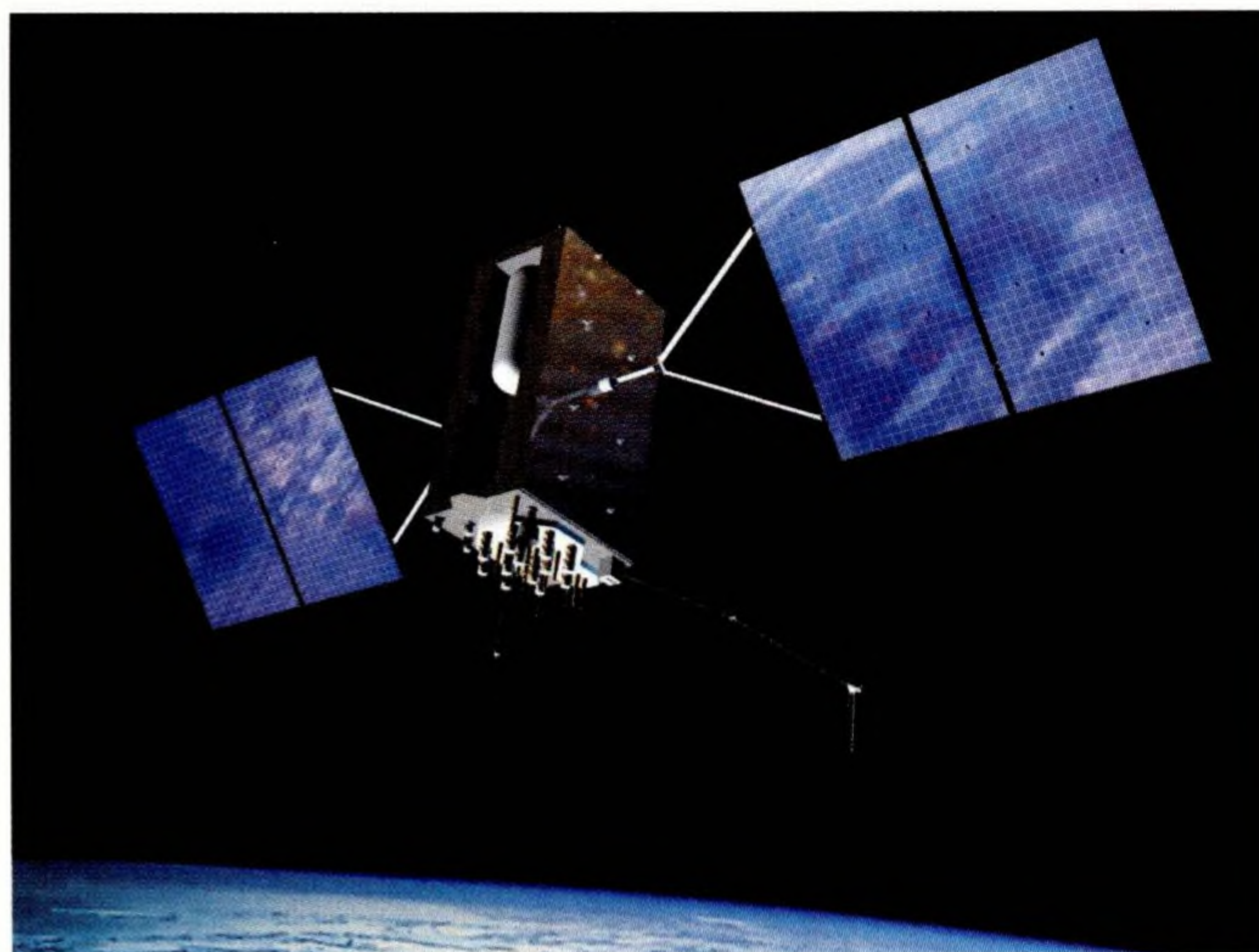
(Above and opposite): an artist's impression of the latest generation GPS Block IIIA satellite by Lockheed Martin, first launched December 23, 2018. These offer three times greater positioning accuracy than their predecessors, increased signal power and much-improved resistance against jamming. The satellites of the GPS constellation are named NAVSTAR (Navigation Satellite Time and Ranging) with various numbers to identify them. See the video titled "Building the Most Powerful GPS Satellite Ever - GPS III" at: siliconchip.com.au/link/aavj
