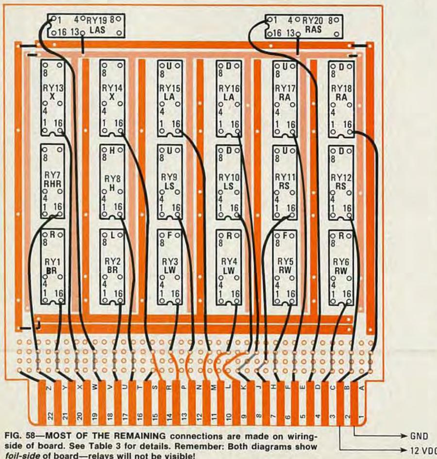
FIG. 58—MOST OF THE REMAINING connections are made on wiring-side of board. See Table 3 for details. Remember: Both diagrams show foil-side of board—relays will not be visible!
