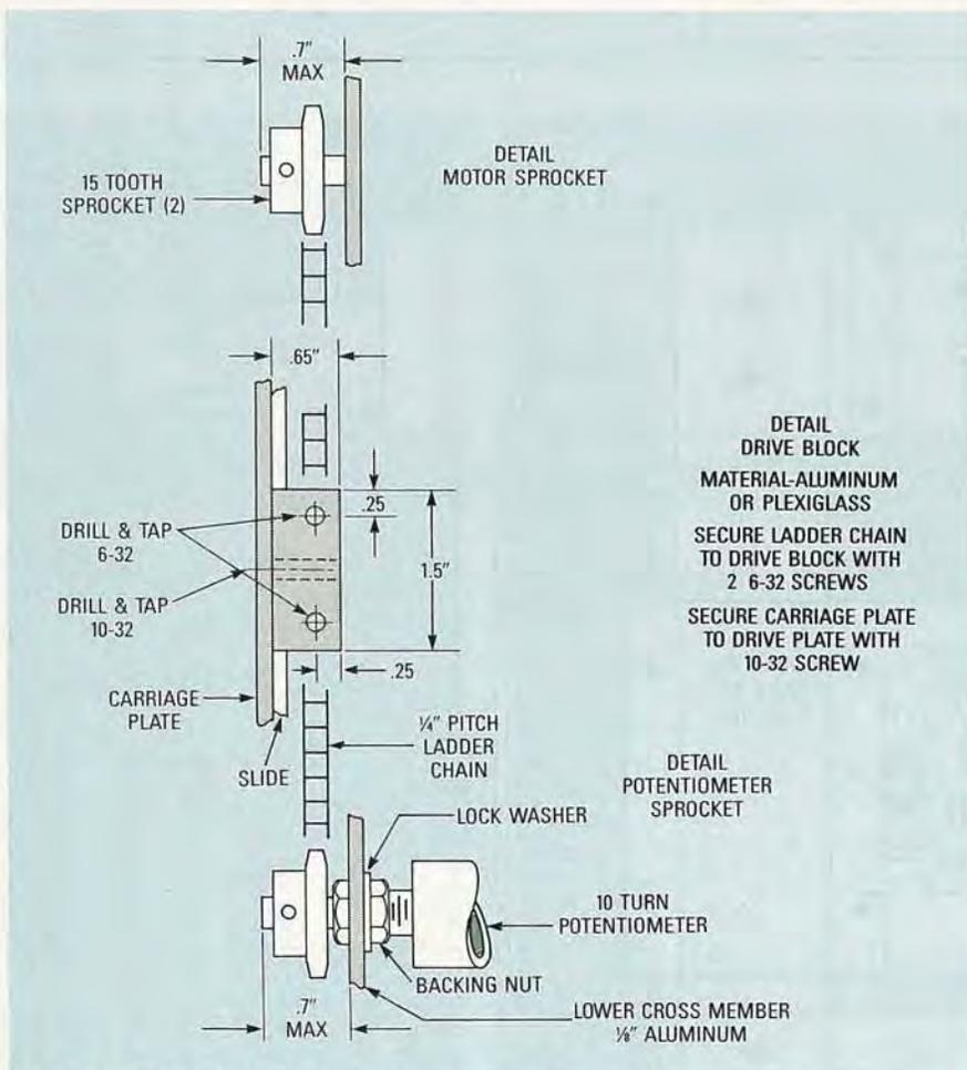
FIG. 3—THIS DETAIL DRAWING shows the ladder-chain drive system.
