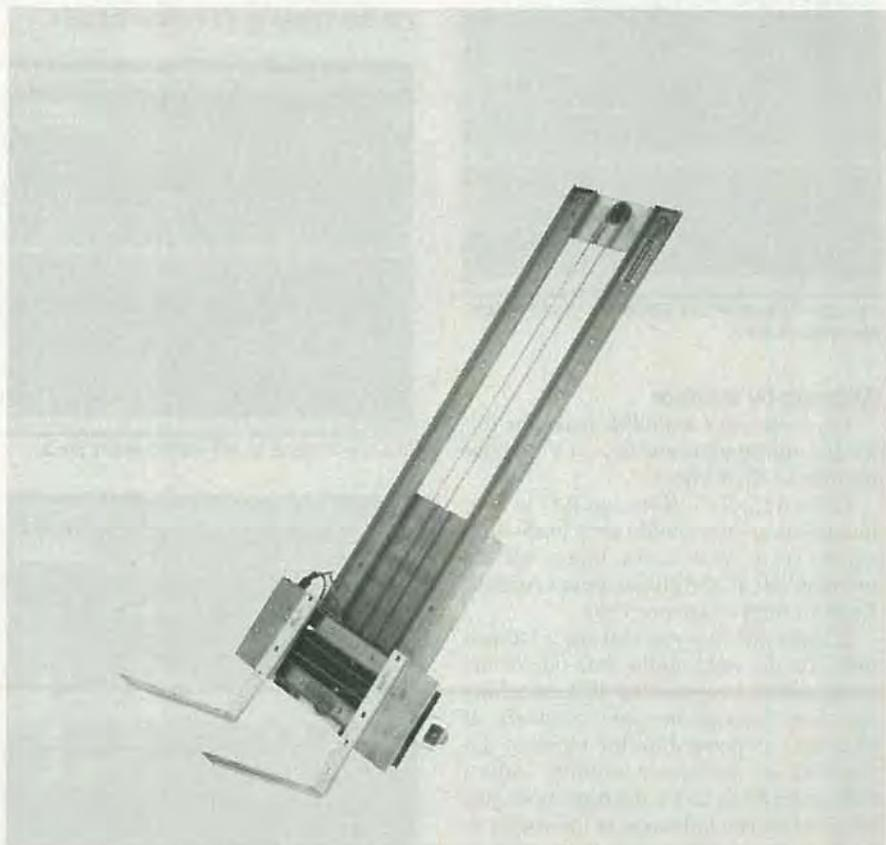
FIG. 1—THIS FORK-LIFT DESIGN can do almost as much as a multi-jointed arm, but with higher lifting capacity and at a lower cost. For greater dexterity, the pincher shown can be added. That pincher, part of which is shown here, will be described in detail in an upcoming installment of this series.
