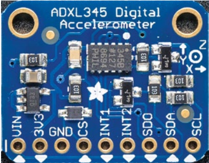
Fig. 4: Pin details of a typical ADXL345 module
