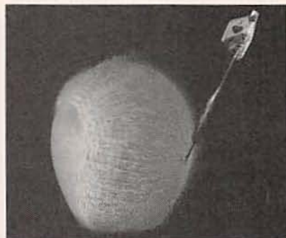
FIG. 5—A DART HITTING a water-filled balloon from an angle. The microphone sensor picked up the sound of the balloon bursting.
