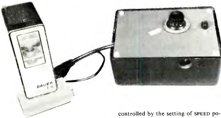
Fig. 1. Schematic diagram (above) of the basic Poor Man's Strobe. Below, a photograph of the author's prototype. The large control knob determines delay between trigger pulse and actuation of flash.
