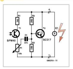
The pulse is transmitted via C1 to the transistor, which then briefly shorts the contacts on the slave gun together. The sensitivity of the device can be adjusted using P1. The circuit can be connected to the shoe contacts of the slave flashgun using a coaxial cable, or, with space permitting and a nimble bit of DIY, can be built inside it.
