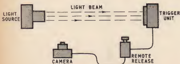
Fig. 1. Diagram of the camera trigger set-up
