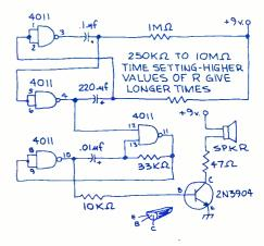
Try connecting +9 volts to pin 14, and the return to pin 7. It's very common to show voltage supply terminals at several points in a diagram. This is done to simplify the drawing by eliminating the need for a single supply line snaking around the circuit. In most circuits, you can assume the ground to be the power supply return. Unless a particular kind of component is specified, you can use anything you'd like with the required rating. Your choice of speaker is fine.
