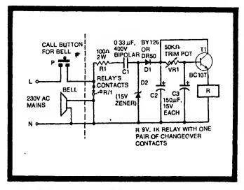
And if the call button is pressed for less than the pre-fixed time, the circuit does not interfer at all.
