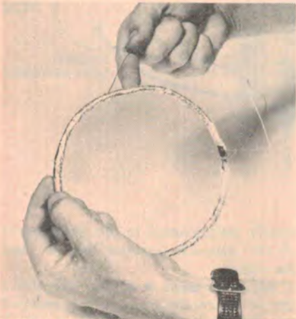
3: Wind tinned copper wire over the shield, passing the end out where the coil leads pass out.
