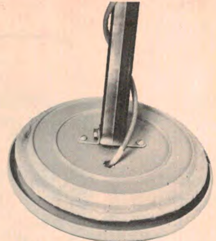
5: Press the assembled coil into the rim of the pot stand, terminate the wires as described and epoxy the coil to the pot stand.
