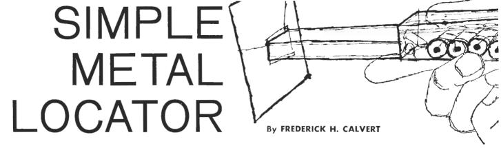
A novel, 1-transistor circuit that will locate wiring and sheet-metal ducts in walls, floors, and ceilings.
